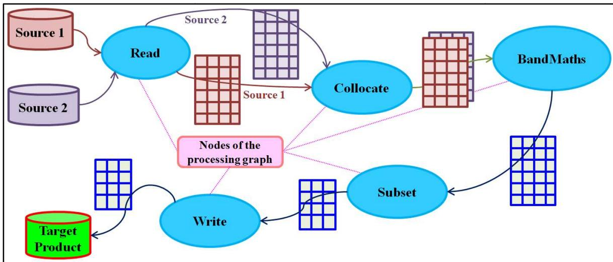
**Fig. 4.3.1: A processing graph comprising five nodes. Graph pull-processing is triggered by the "Write" operation requesting raster data from its source node.**
