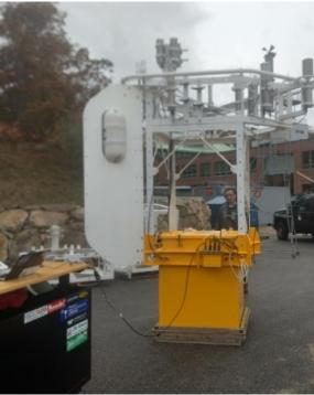
ASIMET Data Logger in the Buoy well and Buoy under Spin test.
