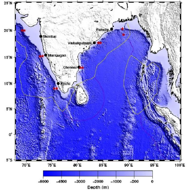
Fig. 5— Locations of ADCP moorings deployed around the Indian coast. At each location, two ADCPs were deployed one at the mid shelf (around 100 m water depth) and the other at the continental slope region (around 1200 m water depth).
