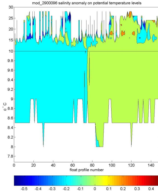
Figure 10: Salinity anomaly plot: Indicates that salinity sensor started drifting from about 65<sup>th</sup> profile.
