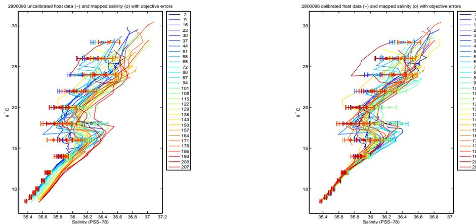
Figure 8: Pre - Calibration(left) & Post Calibration(right) TS diagrams, scatter at close to the bottom indicate clear case of sensor drift, which is rectified in right figure
