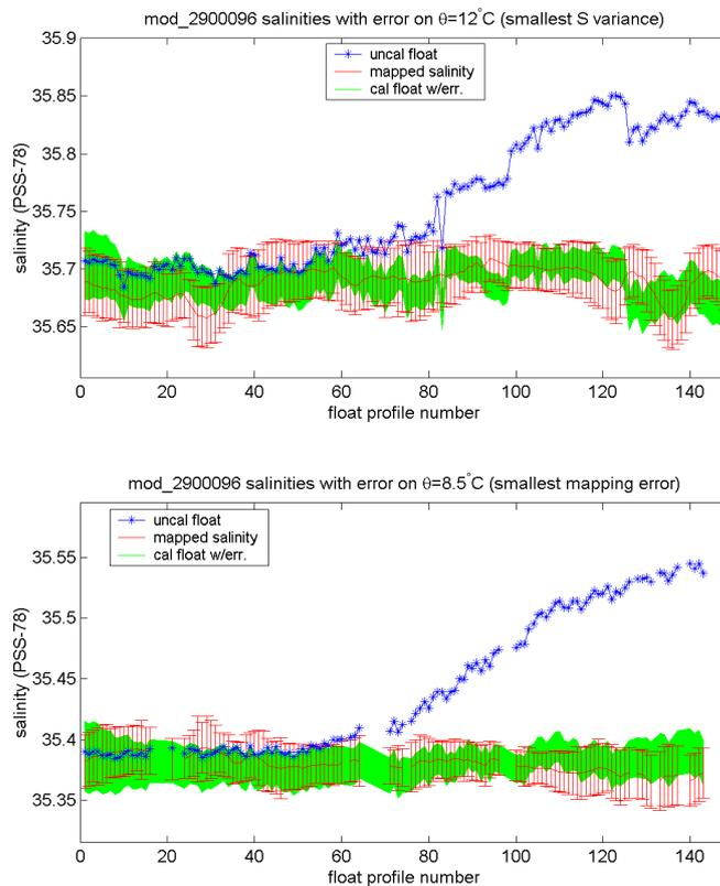
Figure 11: Salinity anomaly plot: Indicates that salinity sensor started drifting from about 65<sup>th</sup> profile.
